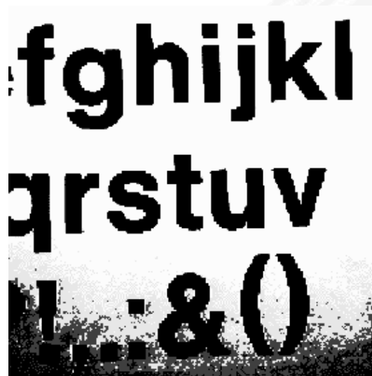
threshold too low
